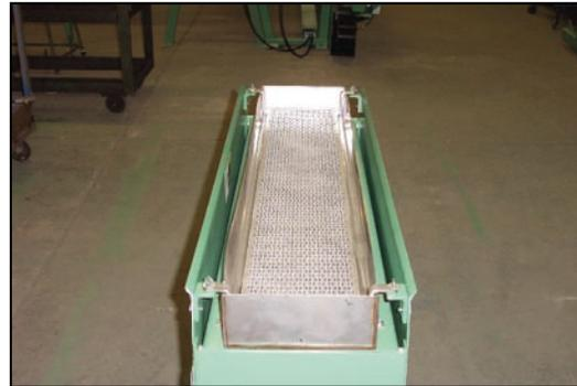
Plate Spreader. Inset: glue spread from Plate Spreader
